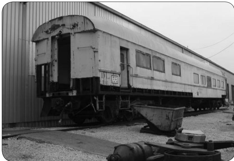
*Diner 741 at Midwest Locomotive on Jan. 16, 2006. All of the rusted areas of the side sheets have been removed, and repairs continue on the side-support beams. (Photo by Michael Steinberg.)*
