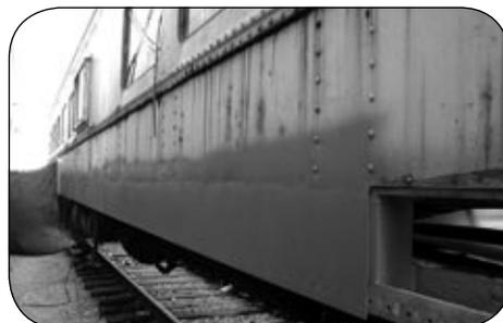
*New side sheets installed on the hallway side of Diner 741 on Feb. 24, 2006. (Photo by Midwest Locomotive.)*
